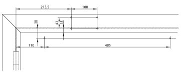
4 - Mounting on frame hinge side
